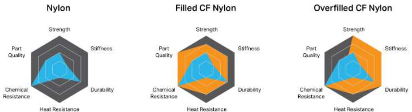
Figure 26: Comparison of properties of Nylon, Filled CF Nylon and Over-filled CF nylon. [27]
