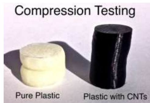
Figure 39: Compression test on Pure ABS and ABS material having CNT infused in it. [47]
