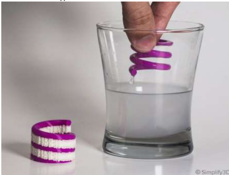
Figure 15: Final product after using PLA as the support structure [19].
