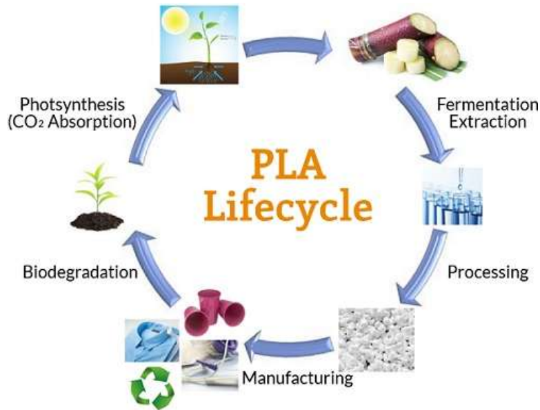
Figure 14: PLA extraction process. [17]
