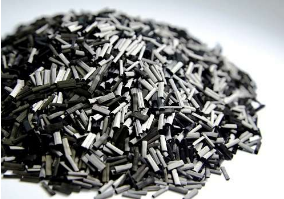
Figure 24: Chopped Carbon fiber to be added to thermoplastic. [30]
