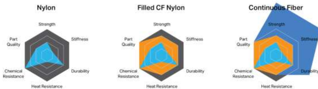
Figure 28: Comparison of properties of Nylon, Filled CF Nylon and Continuous Fiber. [27]
