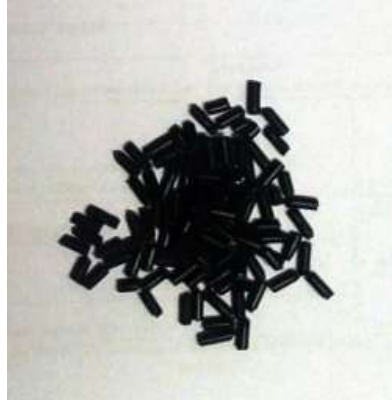
Figure 35: ABS dispersed with MWCNT pellets.[45]
