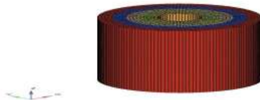
Fig.2. FE Model of the Exhaust manifold section
