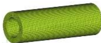
Fig.4: FE Model of Silica insulation Table.7. Meshed result of SILICA section
