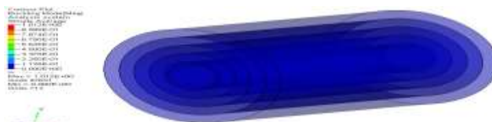
Fig.15: Buckling plot for the exhaust manifold section
