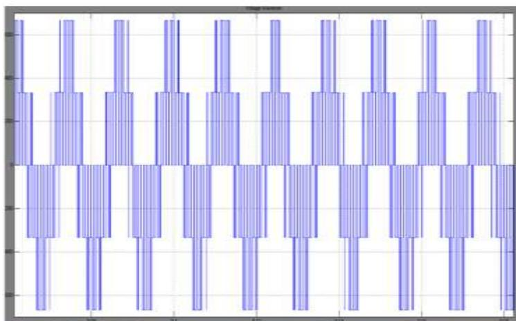
Fig.7 Five level output phase voltage waveform
