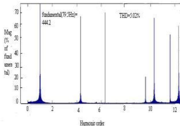
Fig.6.Spectrum of the phase voltage waveform
