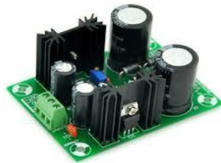
Fig. 4.2 Power supply board
