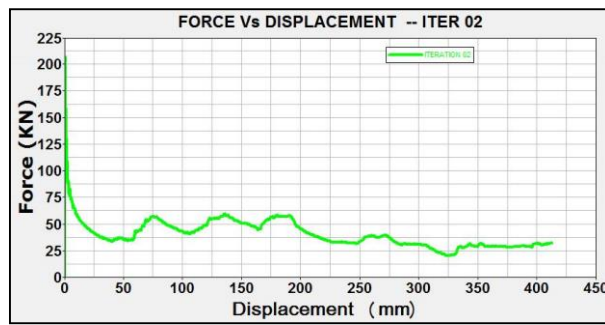
Figure 26: Force Vs Displacement (Energy Absorbed by Material) for Iteration 2
