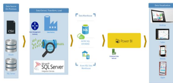
Fig. 1. Azure Data Factory Pipeline Flow [5]
