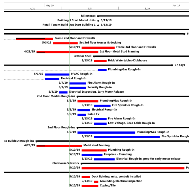
Figure 1: Example of a Gantt Chart showing the tasks in Critical Path (Bar in Red)
