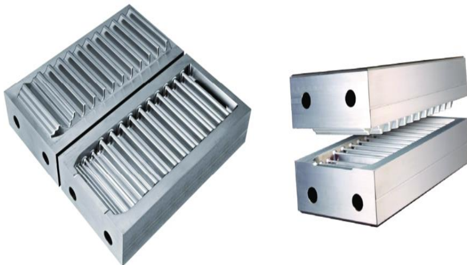
Figure 3.2.2: Chill-vent usage in Die-casting Die
