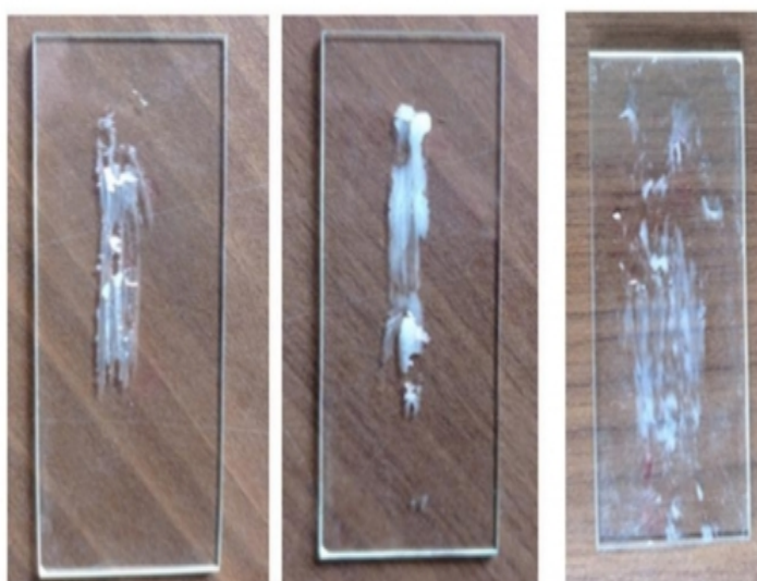
Figure 2: Spreadability of Lip Balm (A) at 25\pm 2^\circ\text{C} , (B) at 40\pm 2^\circ\text{C} , (C) at 5\pm 2^\circ\text{C}
