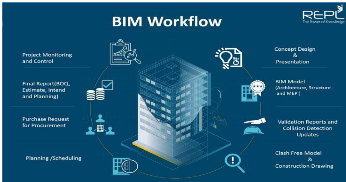
Figure 1: The figure illustrates the BIM Workflow, detailing key stages from concept design and modeling to clash detection, procurement, and final reporting. It emphasizes how BIM integrates various phases of project planning, construction, and monitoring for effective project management.
