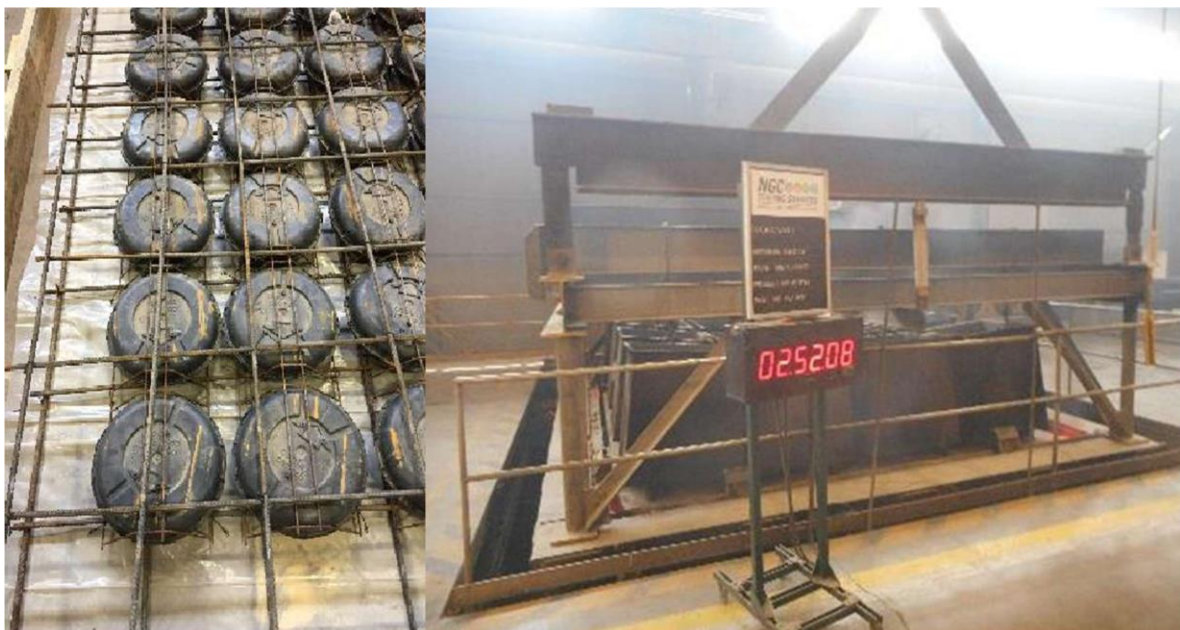
Fire Rating of Voided Slab
