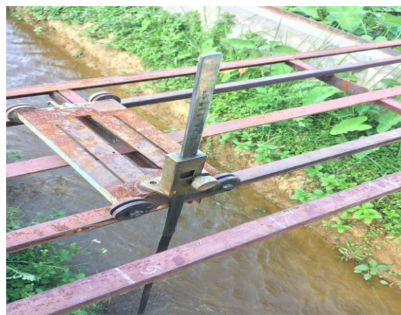
Fig 8: Installed point gauge with steel trolley
