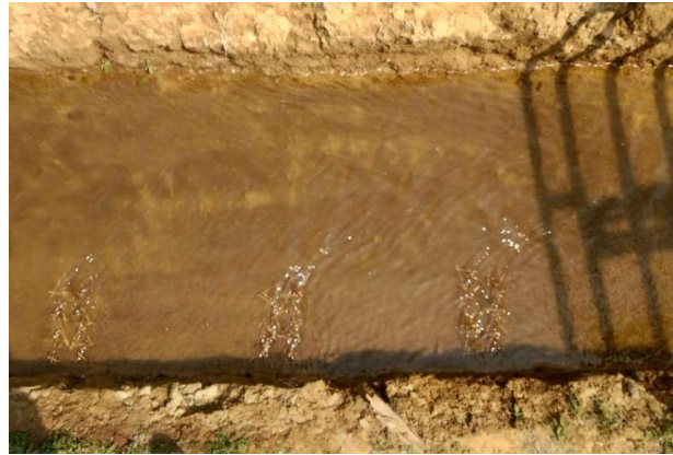
Fig I.1: Channel with installed Porcupine models
