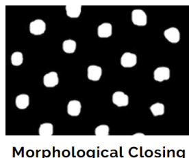
Figure 17: Applying morphological closing to the image
