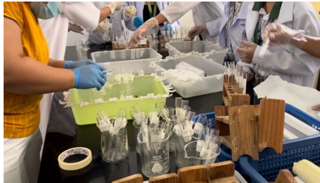
Figure 4: Preparing and labeling the dilution tubes
